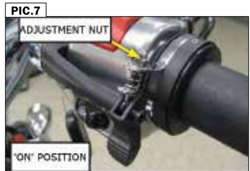
**WARNING** FAILURE TO ADJUST THE MECHANICAL THROTTLE ASSIST PROPERLY MAY RESULT IN LOSS OF CONTROL CAUSING SEVERE INJURY OR DEATH.
