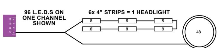
When balancing a branch using Pod Lights the controller reads them as 4 L.E.D.s, but the actual count is 8 L.E.D.s per Pod. The 8 count is used in the overall total of L.E.D.s on a channel. Make sure not to exceed the 100 L.E.D. maximum capacity per channel.
